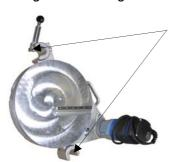
Therefor the eyes must be lubricated with PTFE-spray before transport!
