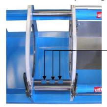
There is a pull-off bar mounted between the movable and the fixed clamping shells on the WI PRECISION basic machine. It prevents the WI HEAT heating element from sticking to the heated-up pipe ends. When inserting the WI HEAT heating element take care
